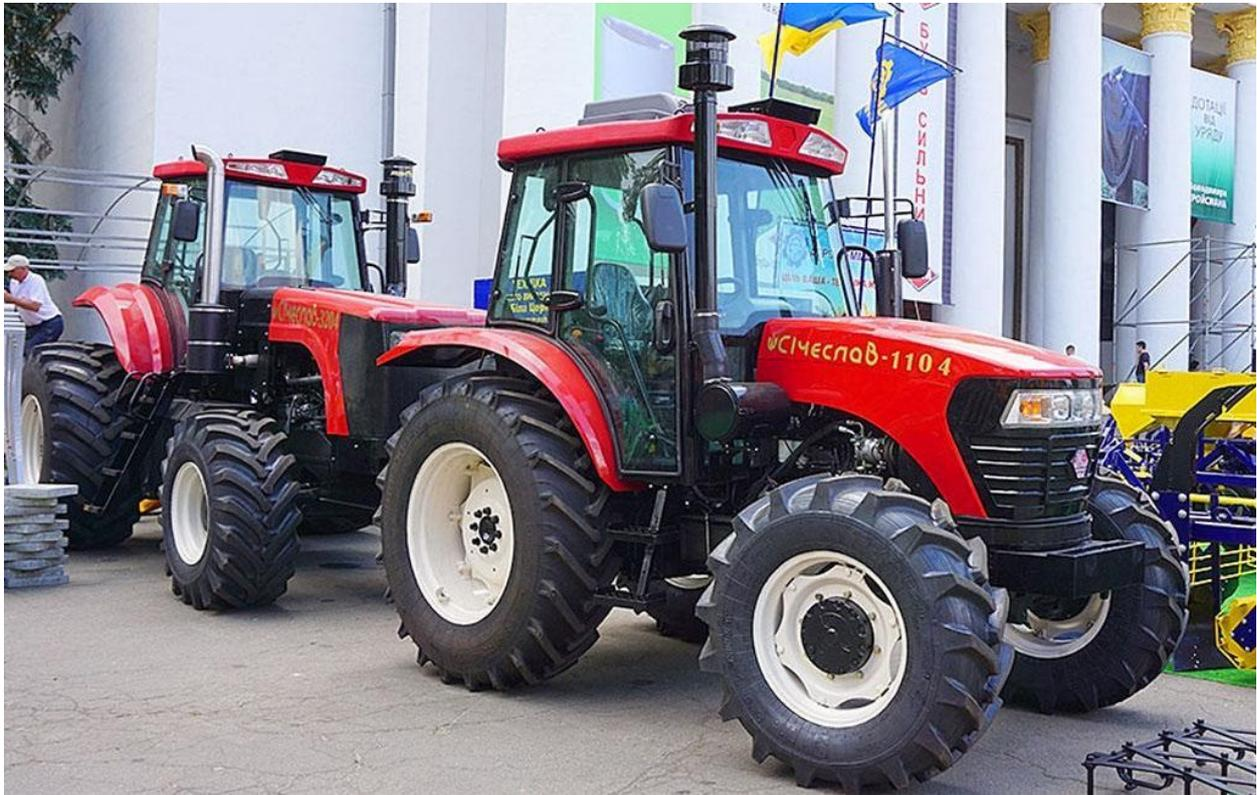
Let's start with the wheeled tractor "**Sicheslav-1104**". It is equipped with 4-cylinder diesel engine Deutz WP4T110E200 with power 110 hp (430 Nm for 1400 - 1600 rpm). Transmission - mechanical, 16 transmission - forward, 8 - back. Fuel consumption - 195 g/kWh. Capacity of fuel tank - 150 l. Total length with front load - 4330 mm, width - 2080 mm, cab height (with air conditioning) - 3120 mm. Road clearance - 380 mm.
